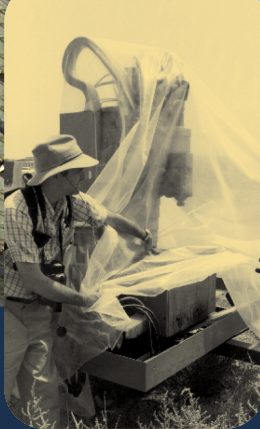
An IAEA Action Team inspector uncovers a Computer-Numerically-Controlled (CNC) machine tool, capable of producing high precision parts, such as for enrichment centrifuges or even nuclear weapons parts, Iraq, IAEA, Action Team, 1991-1998
