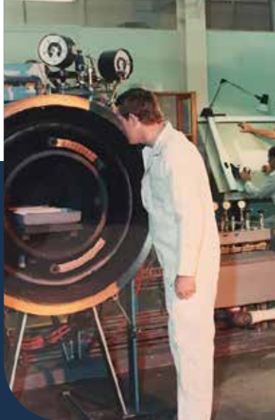
Vacuum induction furnace in circle workshop, Armscor, South Africa, 1990.
