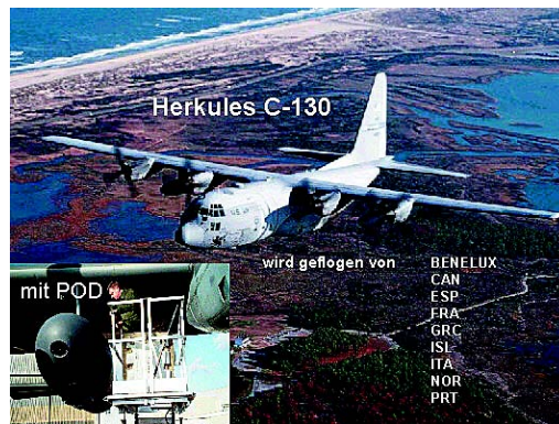
Photo B.5: Image of a Lockheed C-130 Hercules (operated by the Pod Group). Source: German Verification Center, Geilenkirchen. The insert shows the sensor pod mounted under a wing.
