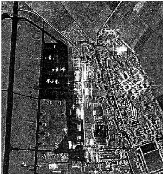
Photo 6.3: SAR image of the military airport at Fürstenfeldbruck, Bavaria, Germany at nominal resolution of 50 centimetres. Photo: Courtesy of Dr. J. Moreira, Aerosensing GmbH, Wessling.
