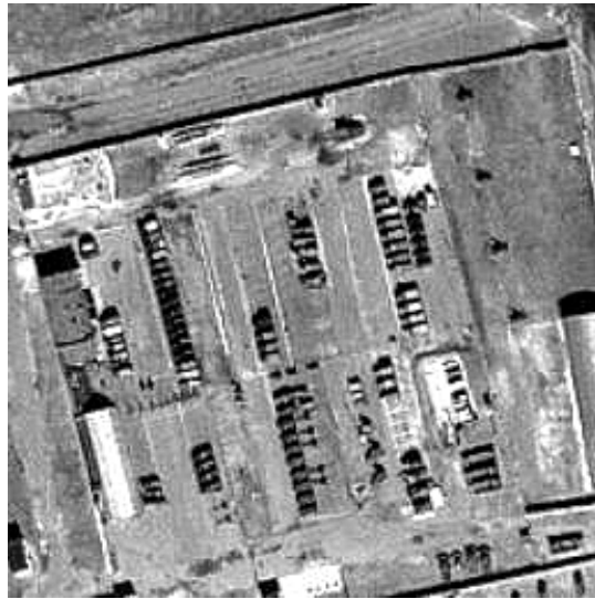
Photo 4.1: Detail of a military vehicle depot at Tiraspol, Moldova. The image was taken by the Ikonos-2 satellite with a ground pixel size of 1 metre, corresponding to a GRD of about 2 metres. Open Skies pictures have superior resolution and recognition potential. Source: H. Spitzer, University of Hamburg.
