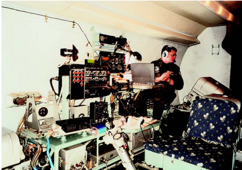
Photo C.2: Camera control electronics on board the Ukrainian Open Skies aircraft. Photo: A. Rothkirch, University Hamburg.
