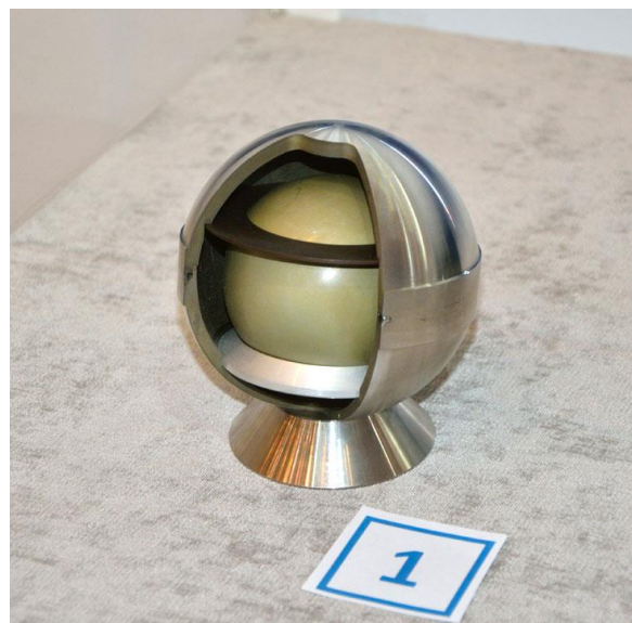
Figure 5. A mock-up of a container that is used to store weapon-origin plutonium at the Mayak Plant Fissile Material Storage Facility
