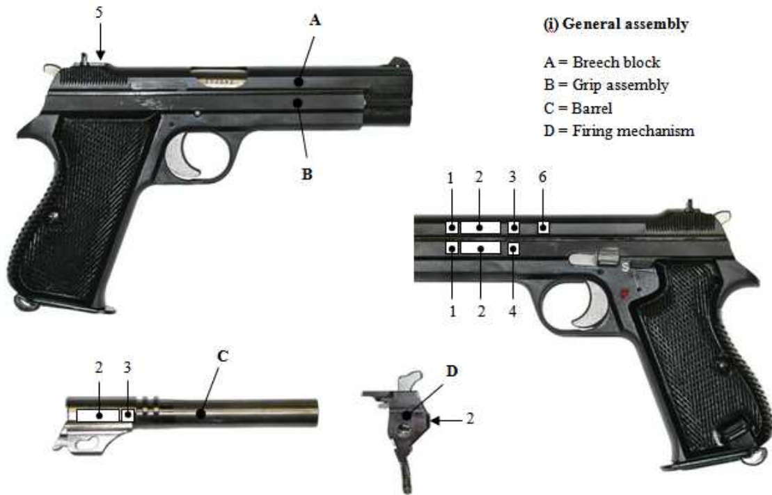
Figure 6. Example of Swiss marking positions and content on a pistol
