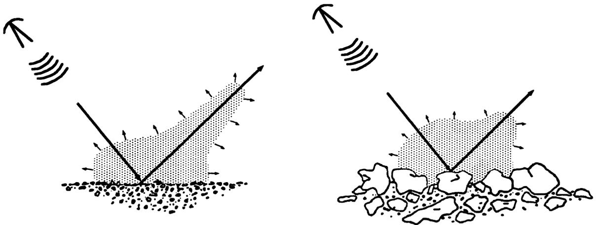
Figure 6.10 Radar backscatter for smooth and rough surfaces. Backscatter from a smooth surface will be characterized by a larger specular component. Backscatter from rough surfaces has a greater diffuse component with little specular reflection. (Redrawn from Robert N. Colwell (editor-in-chief) *Manual of Remote Sensing*, Second Edition, Volume I, p. 1145, © 1983 by the American Society of Photogrammetry and Remote Sensing (ASPRS), by permission of the ASPRS)
