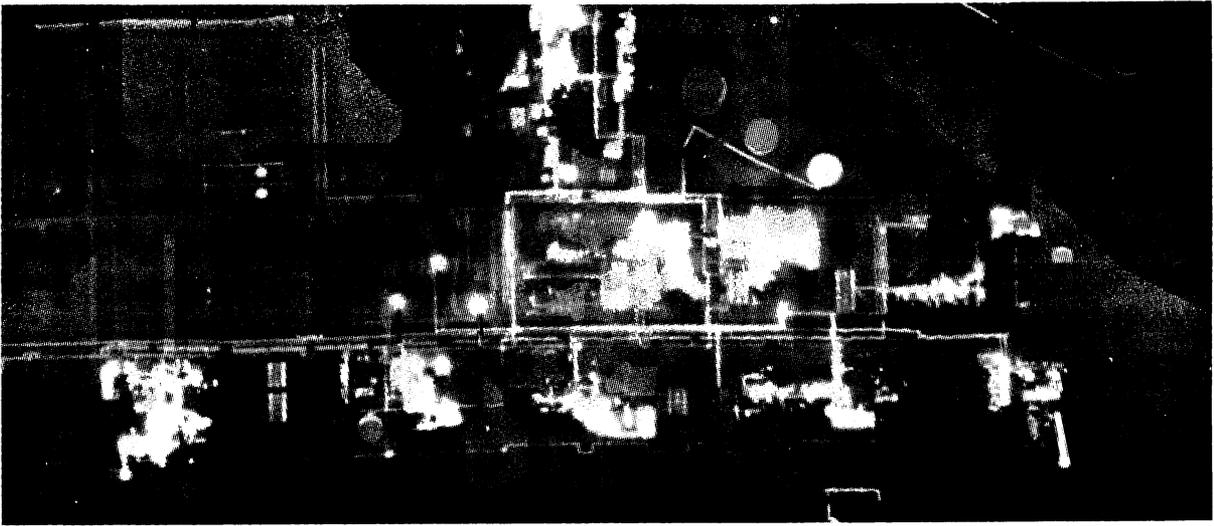
Figure 4.10 The hot targets in this thermal image of an oil refinery may not be as large as they appear. “Blooming” makes hot objects appear larger in size. It takes time for the detector to re-adjust to the relatively low ambient temperature of the background after being boosted by the high radiant temperature of a hot target. (Courtesy of Intera Technologies Ltd.)
