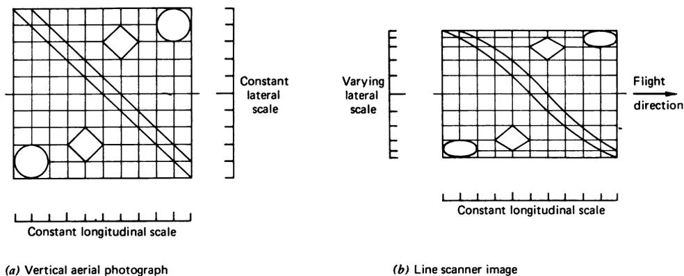
**Figure 4.16** The effects of tangential scale distortion in unrectified linescanner imagery. (From Thomas M. Lillesand and Ralph W. Kiefer, *Remote Sensing and Image Interpretation*, p. 416, © 1979 by John Wiley & Sons, Inc. Reprinted by permission of John Wiley & Sons, Inc., All Rights Reserved.)
