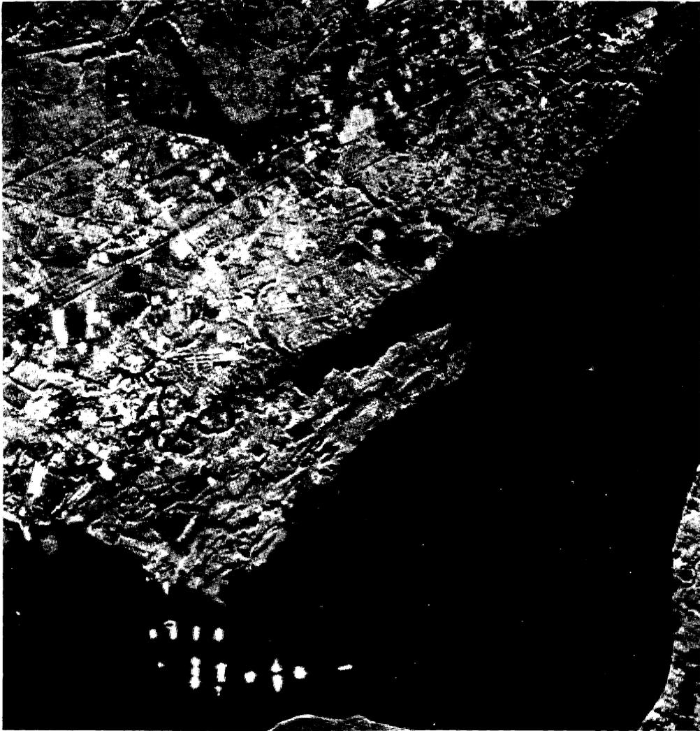
Figure 6.16 The tethered destroyers evident as bright returns near the bottom of this radar image are plainly visible but not necessarily easy to identify. Many common cultural features, such as roads, an airport, and housing subdivisions, are evident. The flight line was oriented parallel to the lengths of the ships to maximize the return from them. (Courtesy of Intera Technologies Ltd.)
