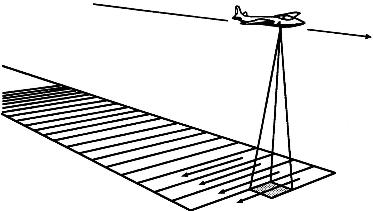
Figure 4.7 Operation of an airborne line scanner to produce contiguous imagery. (Redrawn from Madding, Robert P., "Thermographic instruments and systems." University of Wisconsin-Extension. Department of Engineering and Applied Science, p. 70, © 1979 by the University of Wisconsin Board of Regents, by permission of the University of Wisconsin System, Board of Regents, All Rights Reserved.)
