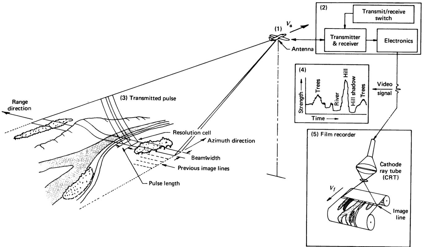
Figure 6.2 Operation of a real aperture SLAR system. (From Thomas M. Lillesand and Ralph W. Kiefer, Remote Sensing and Image Interpretation, p. 495, © 1979 by John Wiley & Sons, Inc. Reprinted by permission of John Wiley & Sons, Inc., All Rights Reserved.)
