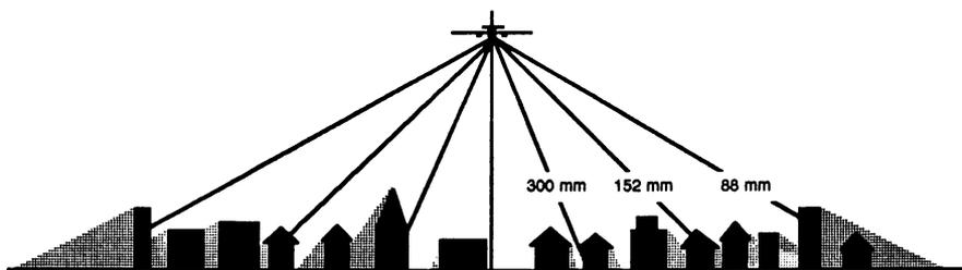
Figure 3.6 Effects of different lens angles on the sizes of dead zones toward the edges of photo frames. (Redrawn from Ron Graham and Roger E. Read, *Manual of Aerial Photography*, p. 215, by permission of Focal Press.)
