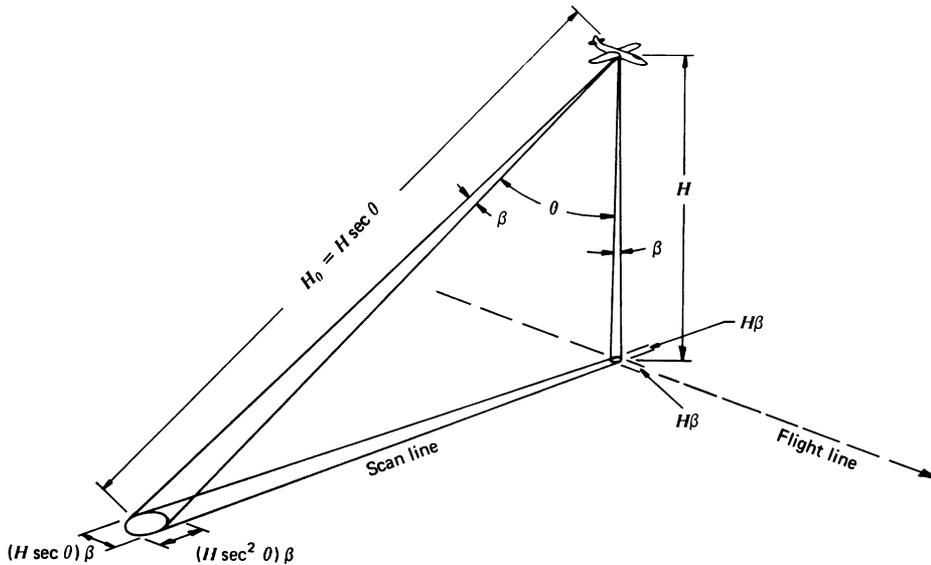
Figure 4.17 Resolution cell size variation with distance from the nadir line. (From Thomas M. Lillesand and Ralph W. Kiefer, Remote Sensing and Image Interpretation, p. 420, © 1979 by John Wiley & Sons, Inc. Reprinted by permission of John Wiley & Sons, Inc., All Rights Reserved.)
