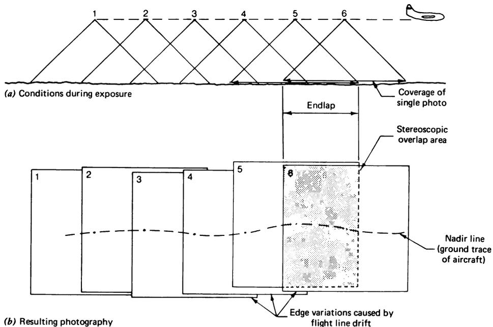
Figure 3.9 Acquisition of overlapping photographic coverage along a flight strip to provide stereoscopic coverage. (From Thomas M. Lillesand and Ralph W. Kiefer, Remote Sensing and Image Interpretation, p. 78, © 1979 by John Wiley & Sons, Inc. Reprinted by permission of John Wiley & Sons, Inc., All Rights Reserved.)
