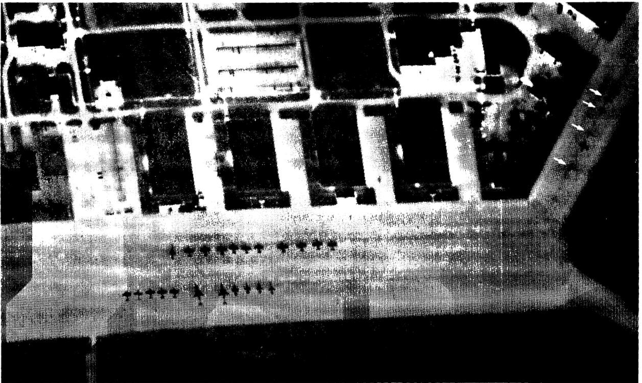
Figure 4.13 Thermal image of a military airfield. Thermal “shadows” of aircraft which were parked on the tarmac during the day are still visible (indicated by arrows) even though the aircraft are no longer there. (Courtesy of Intera Technologies Ltd.)
