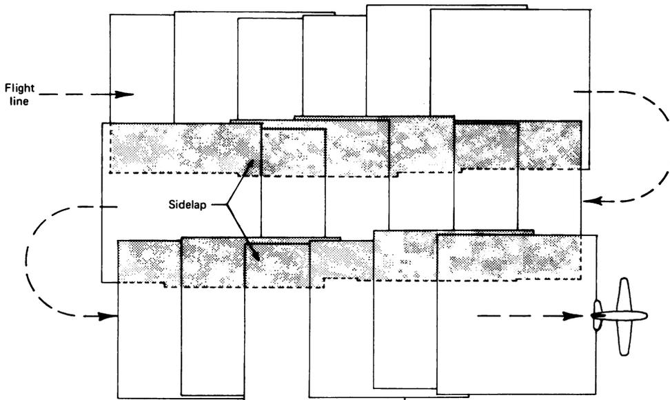
Figure 3.10 The use of sidelap between adjacent flight lines to obtain contiguous coverage of an area. (From Thomas M. Lillesand and Ralph W. Kiefer, Remote Sensing and Image Interpretation, p. 80, © 1979 by John Wiley & Sons, Inc. Reprinted by permission of John Wiley & Sons, Inc., All Rights Reserved.)
