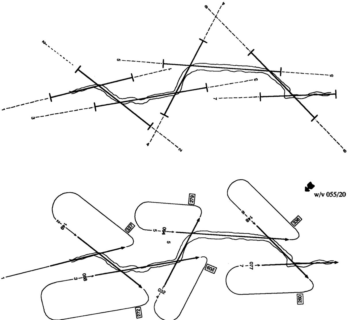
Figure 3.13 Arrangement of flight lines for a feature line survey (top) and the flight pattern to check for crosswinds and drift for each line (bottom). (Redrawn from Ron Graham and Roger E. Read, Manual of Aerial Photography, p. 243 & 244, by permission of Focal Press.)
