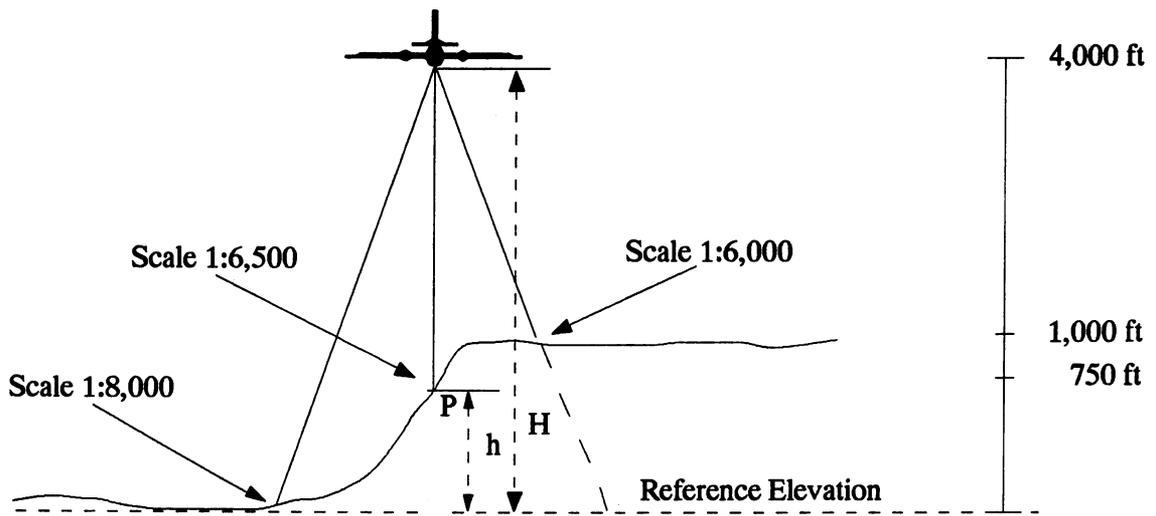
Figure 3.7 Scale and coverage differences over variable terrain. (Redrawn from Ron Graham and Roger E. Read, Manual of Aerial Photography p. 227, by permission of Focal Press.)
