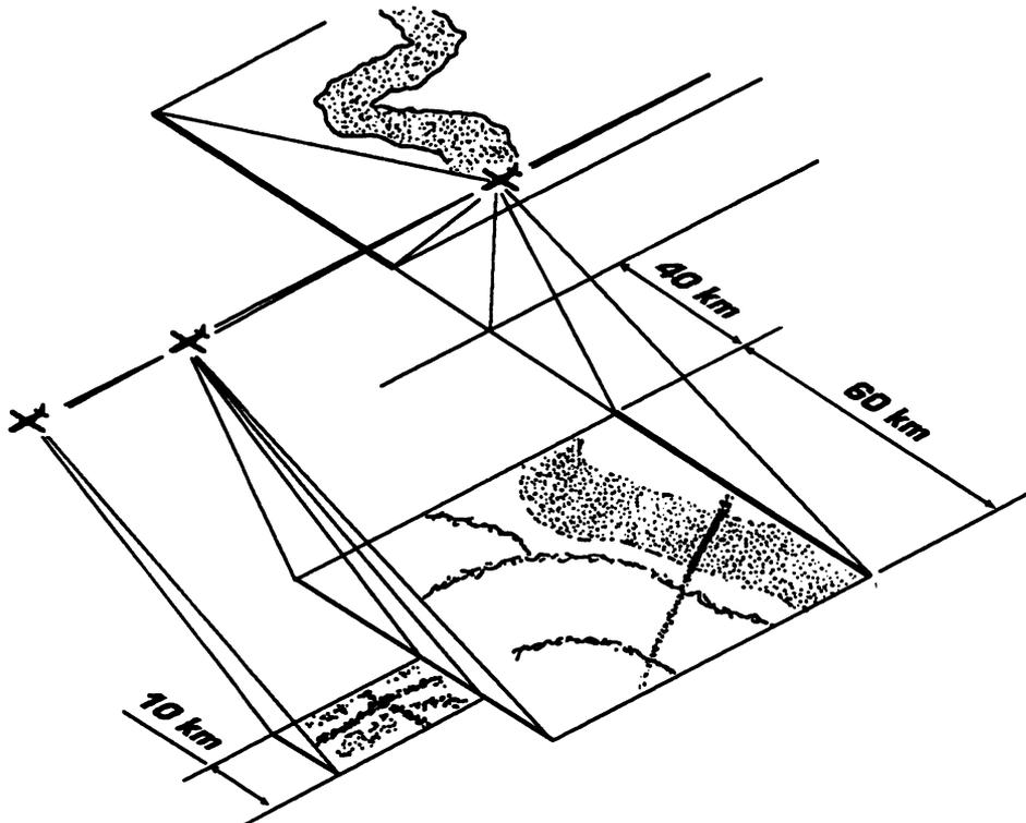
Figure 6.8 Modern stripmap SARs can operate in several modes: a wide-area mode for general surveillance and a high resolution mode for finer detail of smaller areas of interest. They can also be configured to provide a dual-sided capability to maximize the territory which can be imaged in one overpass. (Courtesy of MacDonald Dettwiler and Associates)
