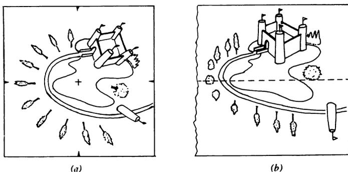
Figure 4.18 Relief displacement in a photograph and in linescanner imagery. In vertical photography, vertical features are displaced radially from the principal point (a). In linescanner imagery, vertical features are displaced at right angles from the nadir line. (From Thomas M. Lillesand and Ralph W. Kiefer, Remote Sensing and Image Interpretation, p. 421, © 1979 by John Wiley & Sons, Inc. Reprinted by permission of John Wiley & Sons, Inc., All Rights Reserved.)
