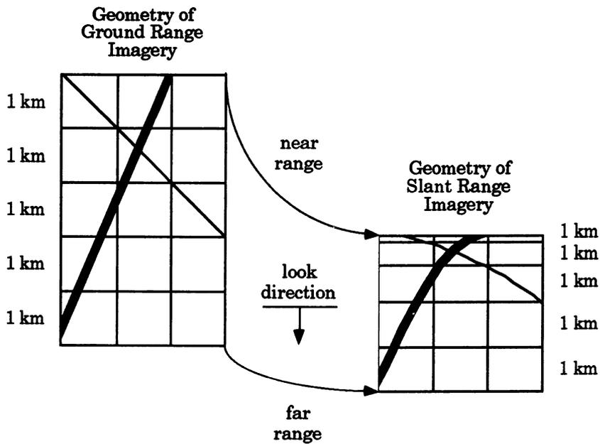
Figure 6.3 Geometry of slant range and ground range presentations. (Redrawn from A.J. Lewis and H.C. MacDonald, "Interpretive and Mosaicking Problems of SLAR Imagery," Remote Sensing of Environment 1 (1970), p. 232, © 1970 by American Elsevier Publishing Company, Inc., by permission of Elsevier Science Publishing, Inc.)
