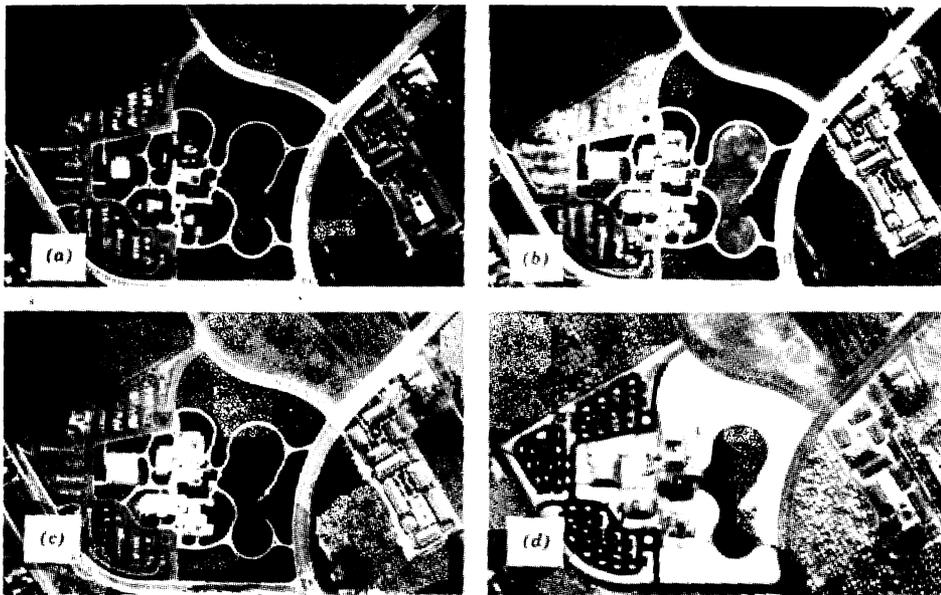
Figure 5.1 Multiband photography taken using black and white infrared film through different filters:
