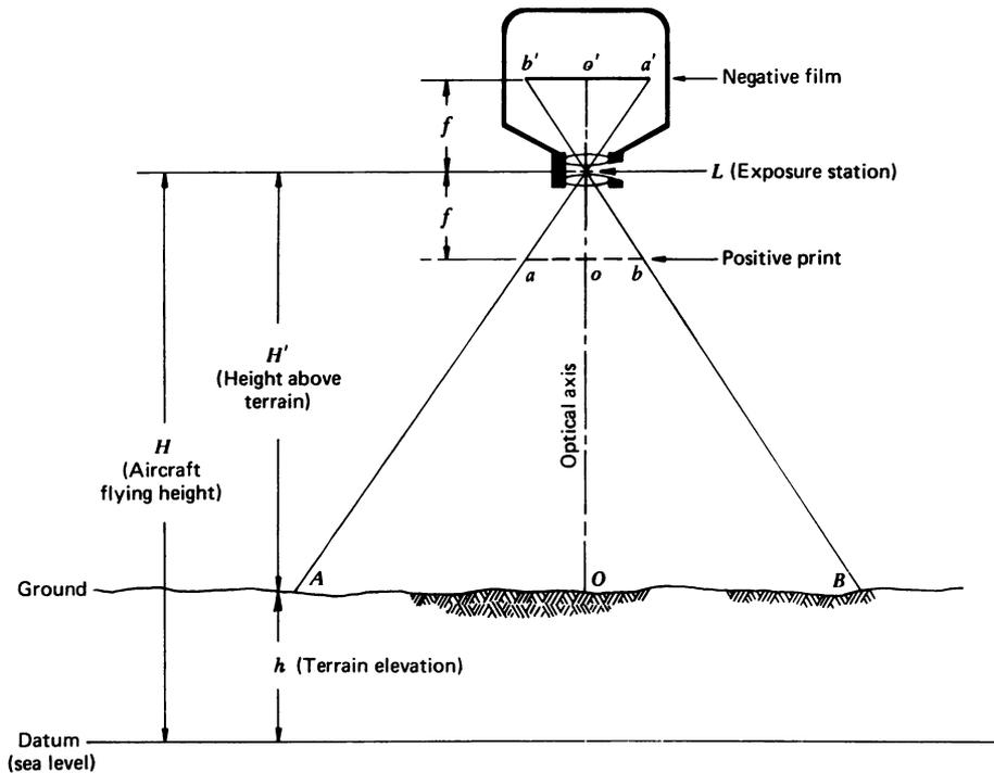
Figure 3.5 Geometric relationships associated with scale calculations for a vertical photograph. (From Thomas M. Lillesand and Ralph W. Kiefer, *Remote Sensing and Image Interpretation*, p. 83, © 1979 by John Wiley & Sons, Inc. Reprinted by permission of John Wiley & Sons, Inc., All Rights Reserved.)
