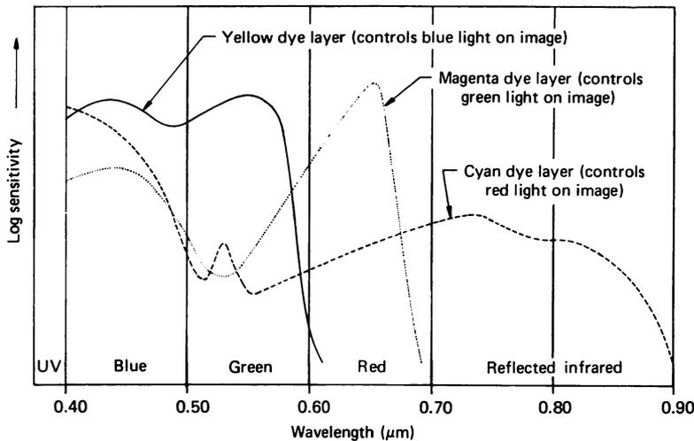
Figure 3.25 Spectral sensitivities for colour infrared film. (From Thomas M. Lillesand and Ralph W. Kiefer, Remote Sensing and Image Interpretation, p. 56, © 1979 by John Wiley & Sons, Inc. Reprinted by permission of John Wiley & Sons, Inc., All Rights Reserved.)
