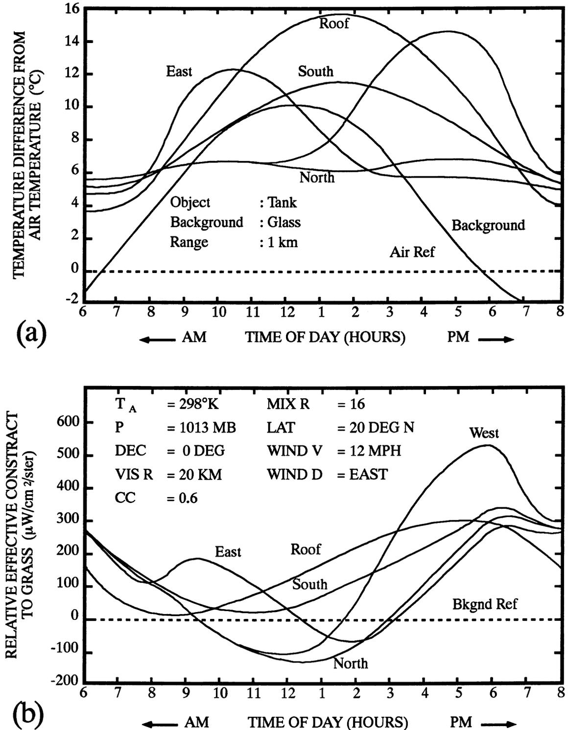
Figure 4.14 (a) Differences between the temperatures of a tank and air, and (b) effective radiant contrast between the tank and a grass background, as a function of time of day for various viewing directions. (Redrawn from Fred Rosell and George Harvey (editors), The Fundamentals of Thermal Imaging Systems. Electro-Optical Technology Program Office, Naval Research Laboratory, Washington, D.C., Report 8311, EOTPO Report No. 46, p. 15-16, by permission of Naval Research Laboratory)
