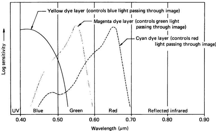
Figure 3.24 Spectral sensitivities for colour film. (From Thomas M. Lillesand and Ralph W. Kiefer, Remote Sensing and Image Interpretation, p. 51, © 1979 by John Wiley & Sons, Inc. Reprinted by permission of John Wiley & Sons, Inc., All Rights Reserved.)
