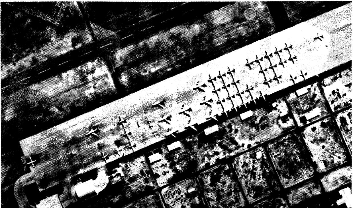
Figure 3.3 Typical vertical panchromatic aerial photograph of an airfield. Several different kinds of aircraft can be distinguished. (Courtesy of David M. Dorschner, Aviation Resource Management)
