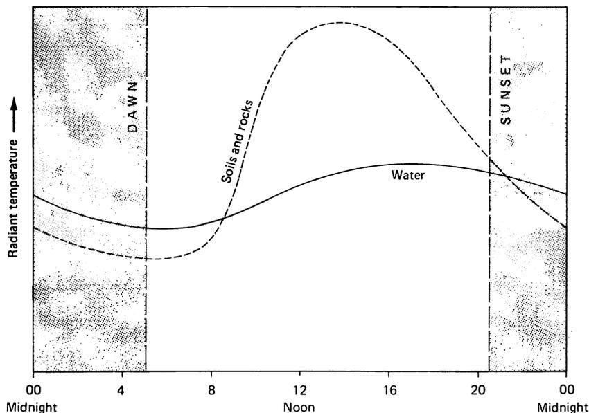
Figure 4.11 Generalized diurnal radiant temperature variations for soils and rocks versus water. (From Thomas M. Lillesand and Ralph W. Kiefer, Remote Sensing and Image Interpretation, p. 403, © 1979 by John Wiley & Sons, Inc. Reprinted by permission of John Wiley & Sons, Inc., All Rights Reserved.)
