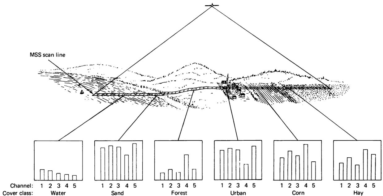
Figure 5.8 Representative multispectral values along one multispectral scan line. The spectral bands represented by the five bars include blue (1), green (2), red (3), reflected infrared (4) and thermal infrared (5). (From Thomas M. Lillesand and Ralph W. Kiefer, Remote Sensing and Image Interpretation p. 459, © 1979 by John Wiley & Sons, Inc. Reprinted by permission of John Wiley & Sons, Inc., All Rights Reserved.)
