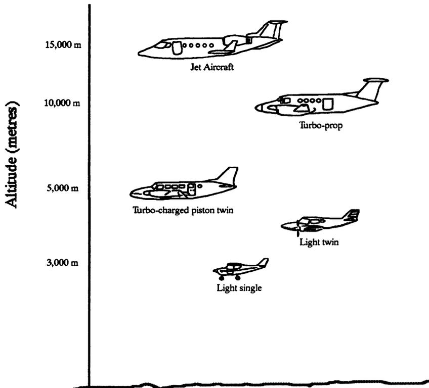
Figure 8.1 Typical operating altitudes for aircraft which might be useful for verification-related overflights. (Redrawn from Ron Graham and Roger E. Read, Manual of Aerial Photography, p. 163, by permission of Focal Press.)
