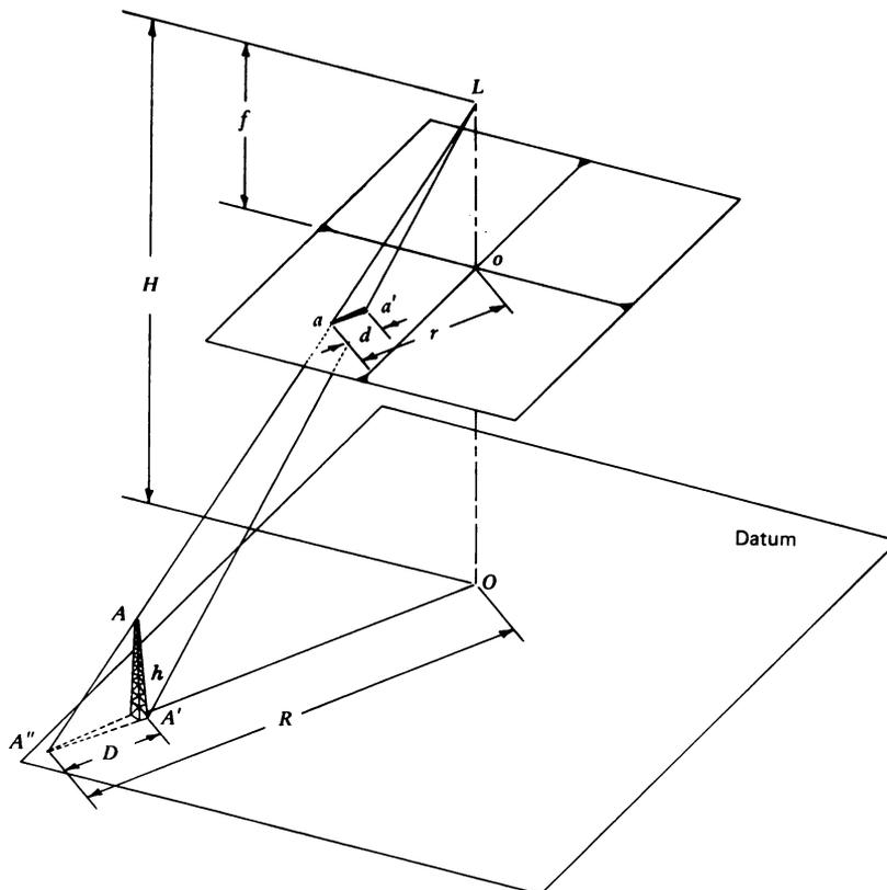
Figure 3.8 Geometric components of relief displacement. (From Thomas M. Lillesand and Ralph W. Kiefer, Remote Sensing and Image Interpretation p. 298, © 1979 by John Wiley & Sons, Inc. Reprinted by permission of John Wiley & Sons, Inc., All Rights Reserved.)
