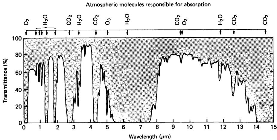
Figure 4.3 Atmospheric transmittance from 0 to 15  $\mu\text{m}$ . The two major windows for thermal sensing are from 3 to 5  $\mu\text{m}$  and from 8 to 14  $\mu\text{m}$ . (From Thomas M. Lillesand and Ralph W. Kiefer, *Remote Sensing and Image Interpretation*, p. 390, © 1979 by John Wiley & Sons, Inc. Reprinted by permission of John Wiley & Sons, Inc., All Rights Reserved.)
