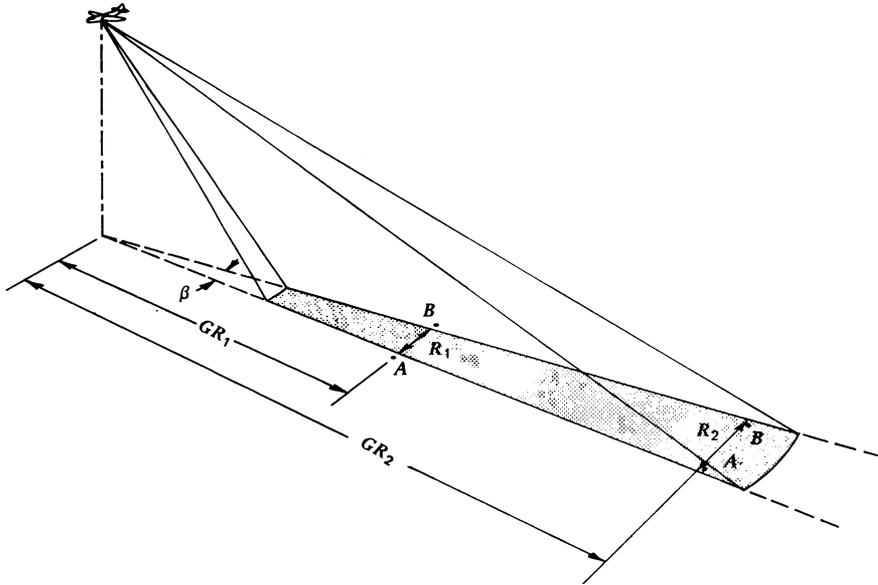
Figure 6.4 Reduction of azimuth resolution ( $R_a$ ) with increasing ground range (GR) for a real aperture radar with beamwidth  $\beta$ . (From Thomas M. Lillesand and Ralph W. Kiefer, Remote Sensing and Image Interpretation, p. 498, © 1979 by John Wiley & Sons, Inc. Reprinted by permission of John Wiley & Sons, Inc., All Rights Reserved.)
