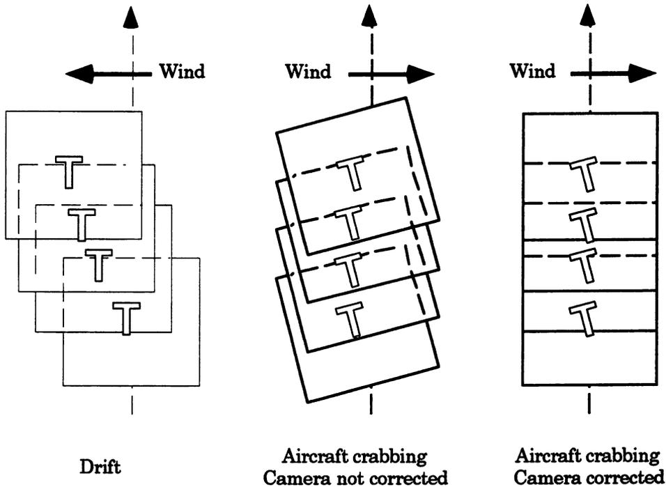
Figure 3.11 Drift is the result of an aircraft being carried off the intended flight line by a crosswind. Crab is the result of the pilot of the aircraft compensating for a crosswind but the camera not being properly oriented to be parallel to the flight line. (Courtesy of Morrie Konick, Consultant, Vinten Military Systems Limited.)
