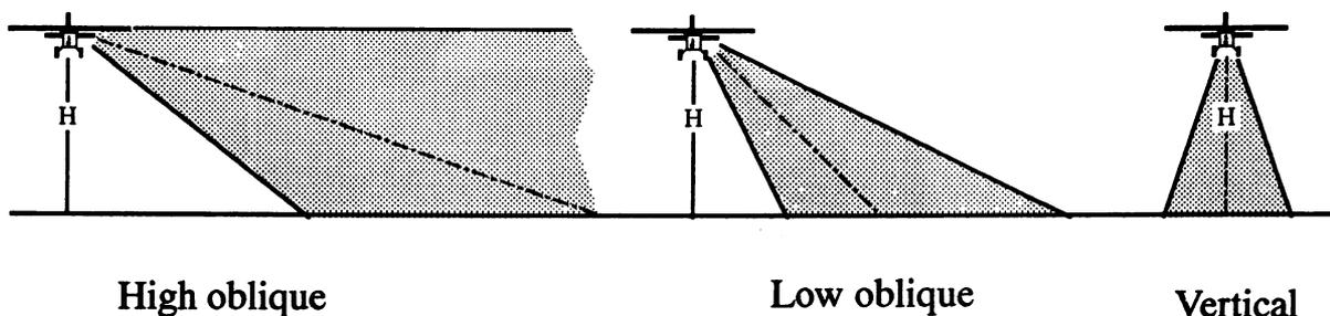
Figure 3.19 Geometries of vertical, low oblique and high oblique photographs. (Redrawn from Barry M. Evans and Larry Mata. 1984. "Acquisition of 35-mm oblique photographs for stereoscopic analysis and measurement." *Photogrammetric Engineering and Remote Sensing* 50(11), p. 1589-90, by permission of American Society of Photogrammetry and Remote Sensing.)
