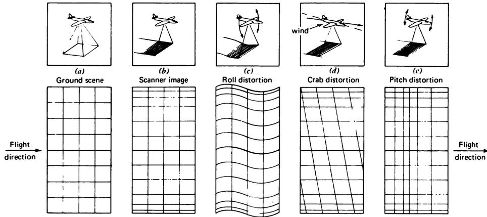
Figure 4.19 Linescanner image distortions induced by aircraft attitude variations. (From Thomas M. Lillesand and Ralph W. Kiefer, Remote Sensing and Image Interpretation, p. 425, © 1979 by John Wiley & Sons, Inc. Reprinted by permission of John Wiley & Sons, Inc., All Rights Reserved.)
