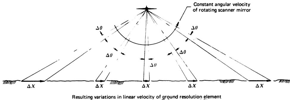
**Figure 4.15** Tangential scale distortion in aerial linescanner imagery is a result of the rotation of the scanner's mirror. (From Thomas M. Lillesand and Ralph W. Kiefer, *Remote Sensing and Image Interpretation*, p. 415, © 1979 by John Wiley & Sons, Inc. Reprinted by permission of John Wiley & Sons, Inc., All Rights Reserved.)
