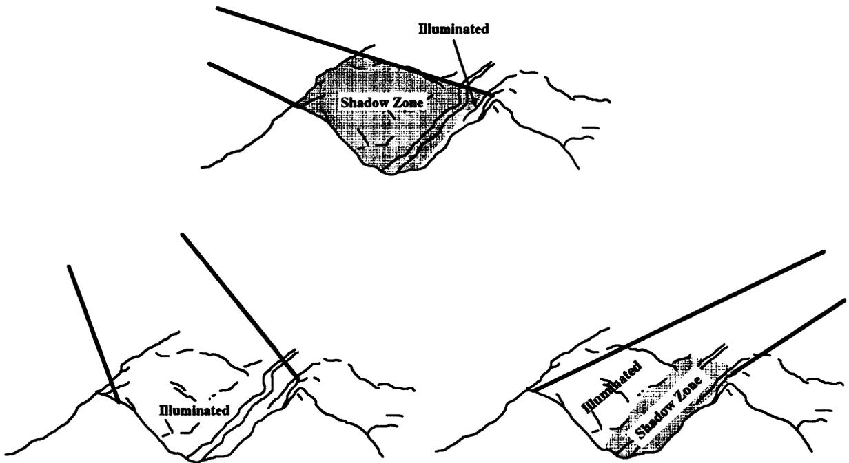
Figure 6.14 Reducing losses of information by radar shadow using overlapping coverage with (a) a steeper depression angle or (b) a different look direction. (Redrawn from L.F. Dellwig et al., "A Demonstration and Evaluation of the Utilization of Side Looking Airborne Radar for Military Terrain Analysis," p. B-8, by permission of U.S. Army Engineer Topographic Laboratories)
