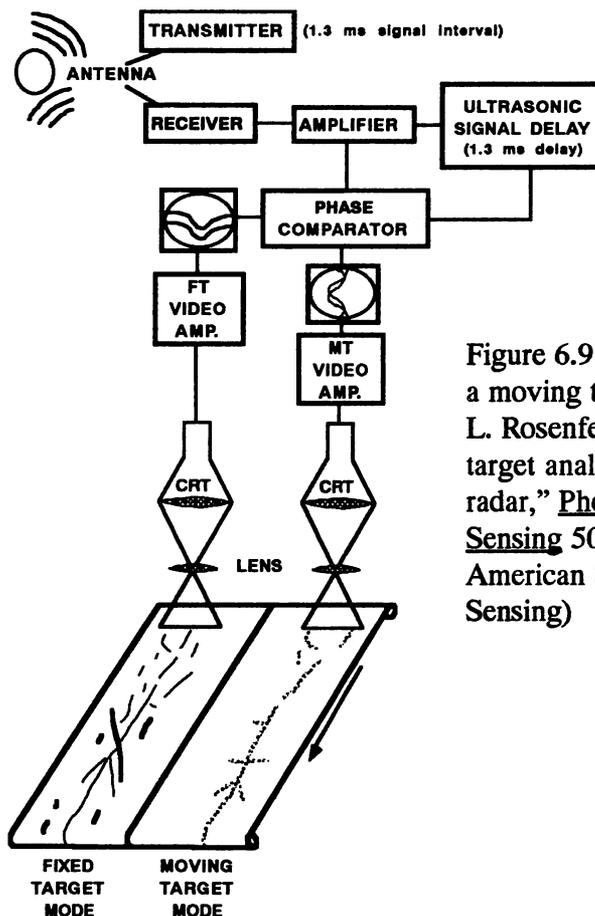
Figure 6.9 Architecture of a SLAR incorporating a moving target indicator. (Redrawn from Charles L. Rosenfeld and A. Jon Kimerling, "Moving target analysis utilizing side-looking airborne radar," *Photogrammetric Engineering and Remote Sensing* 50 (11), p. 1520, by permission of the American Society of Photogrammetry and Remote Sensing)
