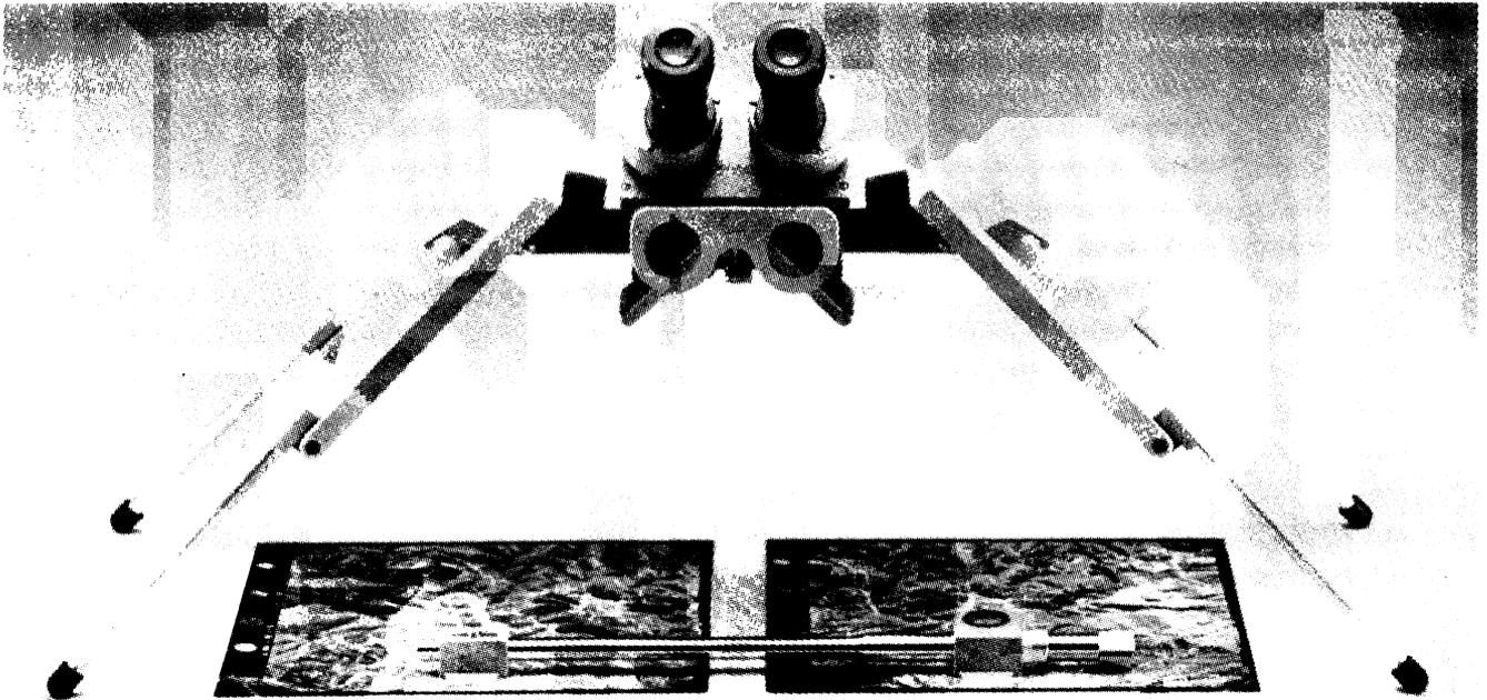
Figure 7.4 Sokkisha MS27 mirror stereoscope with a pair of aerial photographs prepared for stereo viewing and with a parallax bar. (Courtesy of Mark Lystiuk, Currie Engineering, and Sokkisha Co., Ltd.)
