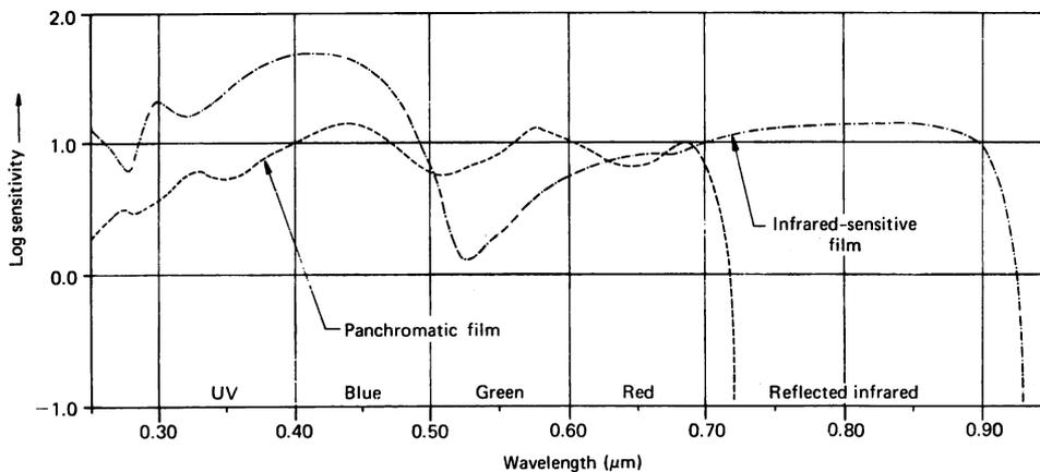
Figure 3.23 Spectral sensitivities for black and white panchromatic and infrared-sensitive films. (From Thomas M. Lillesand and Ralph W. Kiefer, Remote Sensing and Image Interpretation, p. 46, © 1979 by John Wiley & Sons, Inc. Reprinted by permission of John Wiley & Sons, Inc., All Rights Reserved.)
