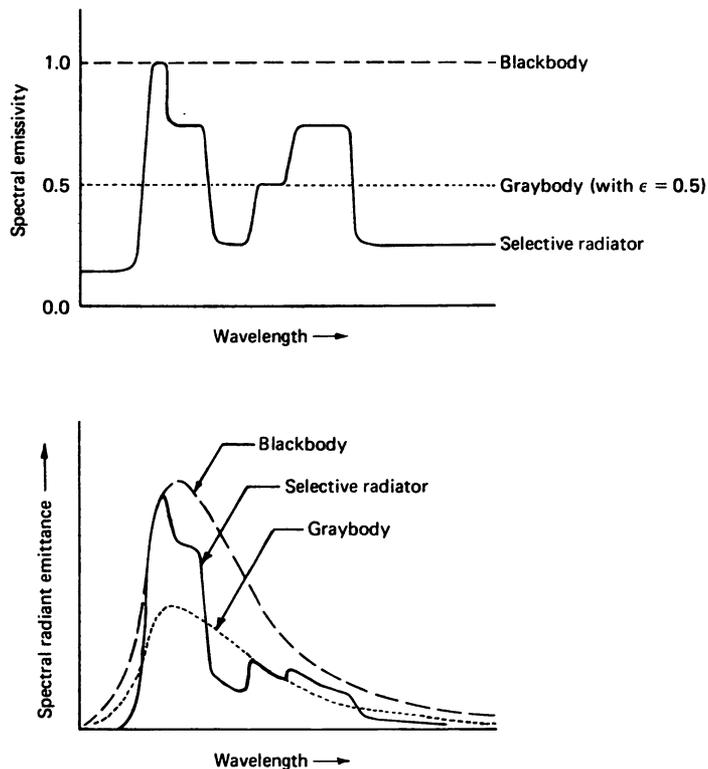
Figure 4.2 Spectral emissivities and radiant distributions of a blackbody, graybody and selective radiator. (From Thomas M. Lillesand and Ralph W. Kiefer, Remote Sensing and Image Interpretation, p. 387, © 1979 by John Wiley & Sons, Inc. Reprinted by permission of John Wiley & Sons, Inc., All Rights Reserved.)
