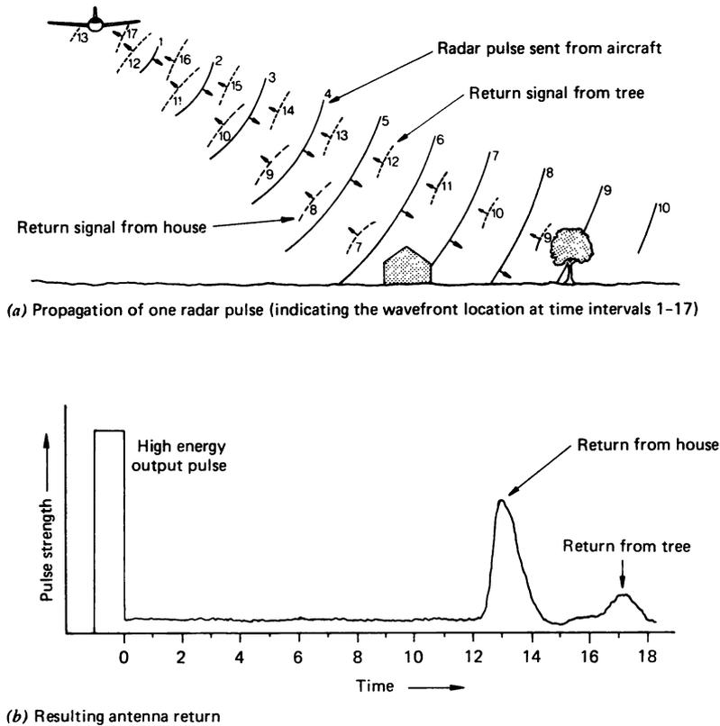
Figure 6.1 SLAR signal transmission and return. (From Thomas M. Lillesand and Ralph W. Kiefer, Remote Sensing and Image Interpretation, p. 493, © 1979 by John Wiley & Sons, Inc. Reprinted by permission of John Wiley & Sons, Inc., All Rights Reserved.)
