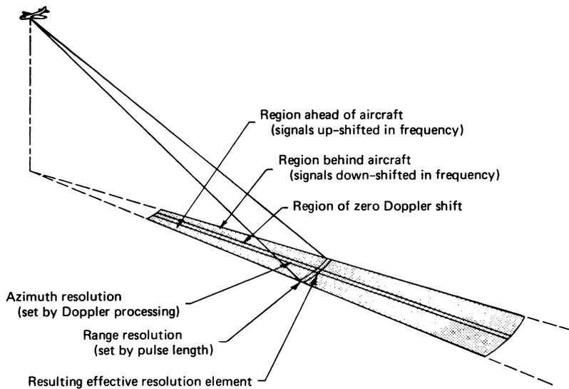
Figure 6.6 Determination of resolution in synthetic aperture radar systems. (From Thomas M. Lillesand and Ralph W. Kiefer, Remote Sensing and Image Interpretation, p. 500, © 1979 by John Wiley & Sons, Inc. Reprinted by permission of John Wiley & Sons, Inc., All Rights Reserved.)
