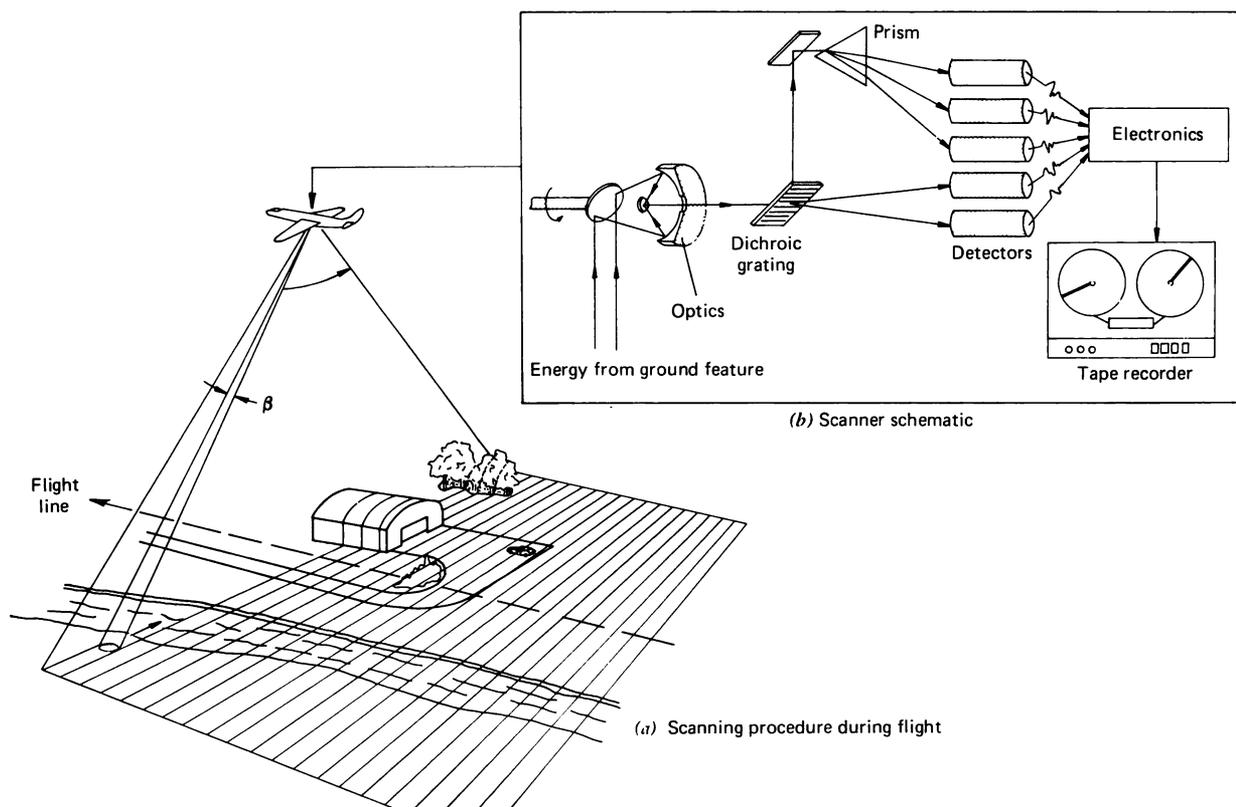
Figure 5.3 Operation of a multispectral scanner. (From Thomas M. Lillesand and Ralph W. Kiefer, *Remote Sensing and Image Interpretation*, p. 444, © 1979 by John Wiley & Sons, Inc. Reprinted by permission of John Wiley & Sons, Inc., All Rights Reserved.)
