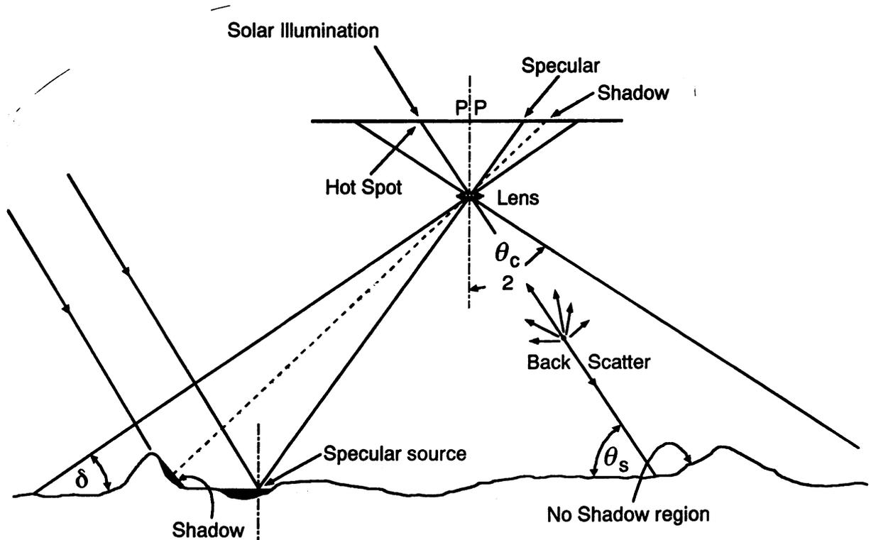
Figure 3.14 Geometry of hot spot and sun spot formation in wide-angle photography. To minimize these effects, flying should be restricted to periods when the solar angle ( $\theta_s$ ) is less than  $\delta$ . (Redrawn from Ron Graham and Roger E. Read, Manual of Aerial Photography, p. 134, by permission of Focal Press.)
