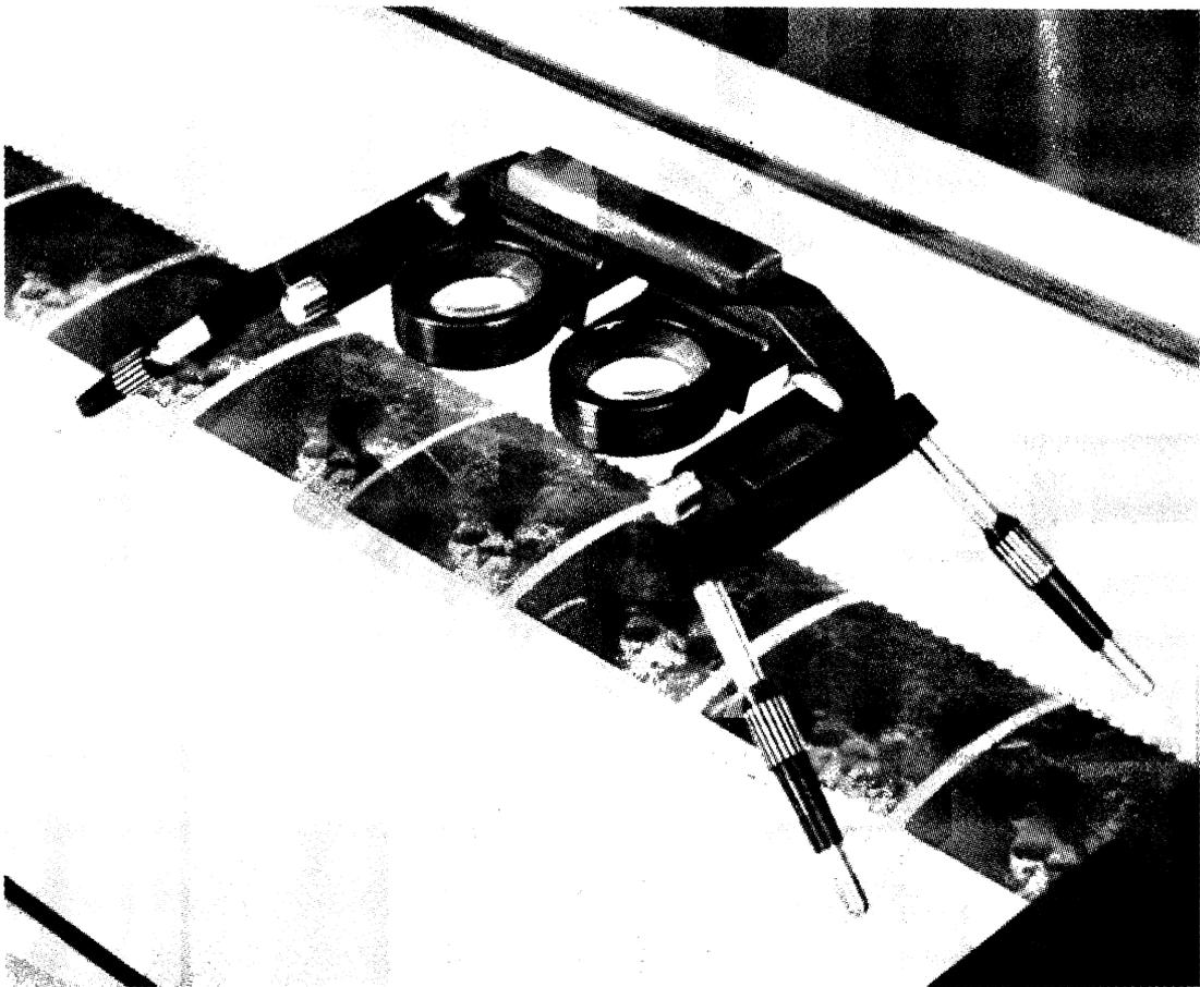
Figure 7.3 Lens stereoscope with 2x and 4x magnification lenses. (Courtesy of Vinten Military Systems Ltd.)
