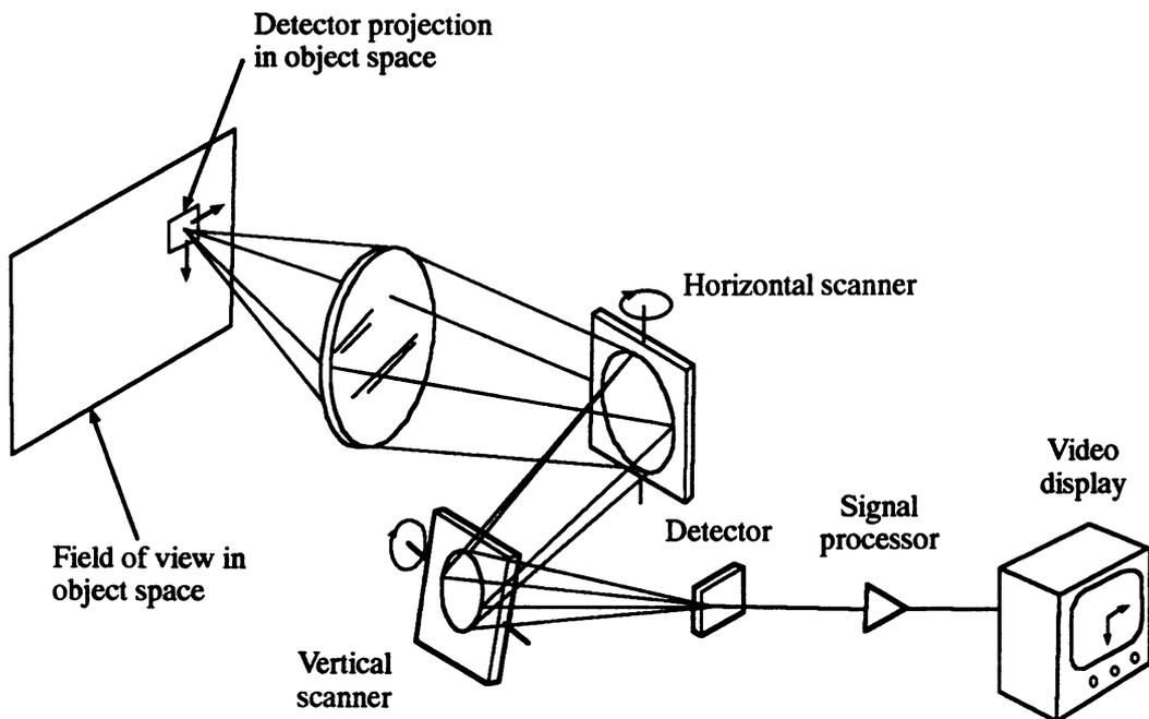
Figure 4.6 Simplified single-detector, dual-axis scanner. An image of the scene is built by focussing thermal energy onto the detector using a two-dimensional (horizontal and vertical) scanning mechanism. (Redrawn from A.L. Rodgers, I.B.R. Fowler, T.K. Garland-Collins, J.A. Gould, D.A. James, and W. Roper, Surveillance and Target Acquisition Systems, p. 80, © 1983 by Brassey's Publishers Ltd., by permission of Brassey's Defence Publishers, Pergamon Press)
