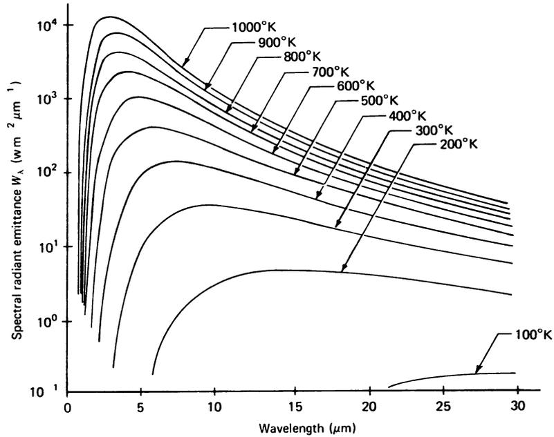
Figure 4.1 Spectral distribution of the energy radiated from blackbodies at different temperatures. (From Thomas M. Lillesand and Ralph W. Kiefer, Remote Sensing and Image Interpretation, p. 385, © 1979 by John Wiley & Sons, Inc. Reprinted by permission of John Wiley & Sons, Inc., All Rights Reserved.)
