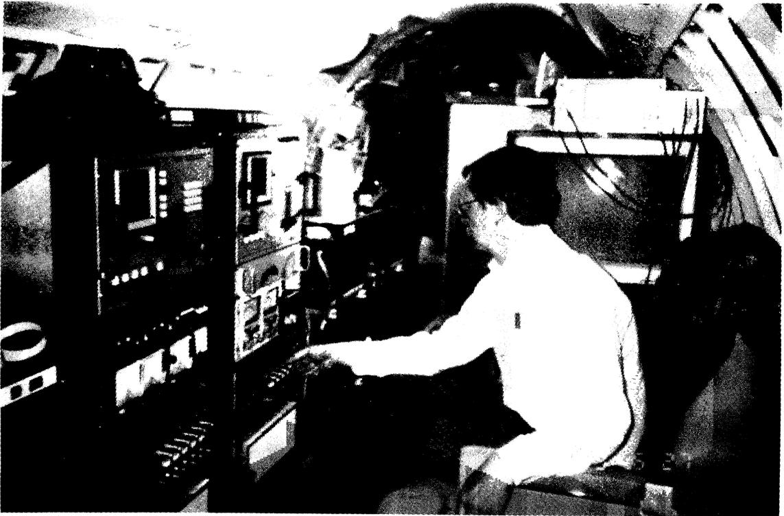
Figure 6.7 Operator at the controls of a SAR with real time, on-board digital processing. (Courtesy of K.L. Link, Intera Technologies Ltd.)
