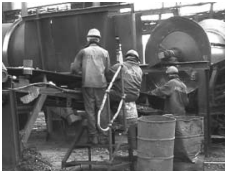
Photo 3: Separation of ferrous and non-ferrous metal during destruction. Photo credit: Institute for Security Studies.
