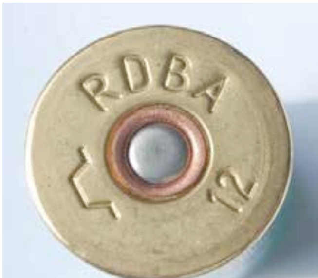
Figure 4: Example of headstamp marking in small arms ammunition in the Dominican Republic. 15
