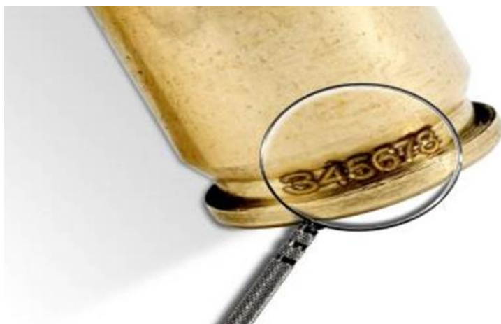
Figure 6: Example of laser markings in small arms ammunition by the Federal Police of Brazil. 17
