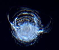
A 7 mm-diameter circular chip in the ISS' Cupola window gouged out by the impact from a tiny piece of space debris, possibly a paint flake or small metal fragment no bigger than a few thousandths of a millimetre across.
