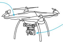
The **payload** refers to additional components which can be carried by the UAS but are not essential to its operability. Both civilian and military vehicles can incorporate a payload. This can include additional sensors (beyond those needed for navigation), goods (e.g., medical supplies or food), or weapons systems.
