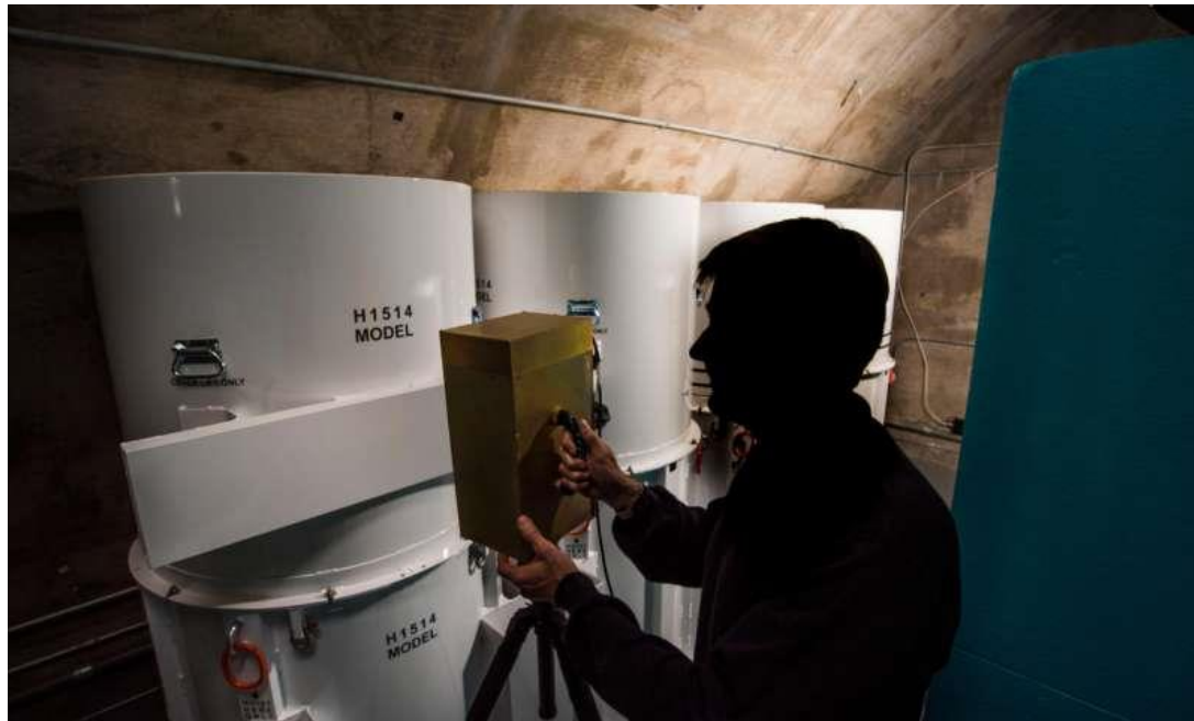
Sandia National Laboratories: new radiation detection equipment being tested for New START monitoring. Source: https://commons.wikimedia.org/wiki/File:INF_inspection.JPG
