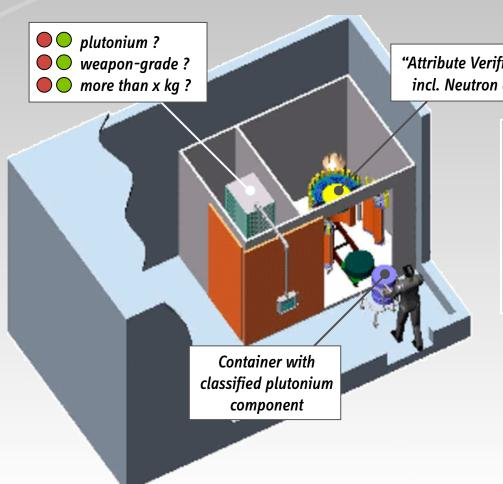
"Attribute Verification System" (AVNG) incl. Neutron and Gamma Detector
