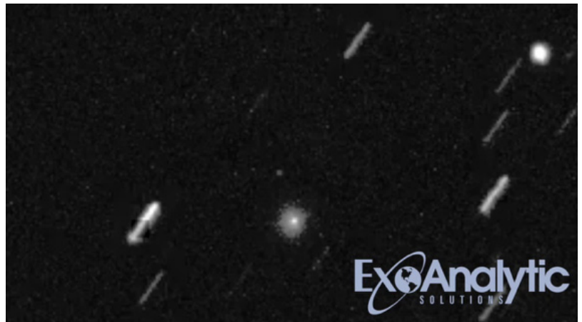
Figure 1: an image of a satellite in GEO, with stars streaking in the background. (Courtesy of ExoAnalytic Solutions)
